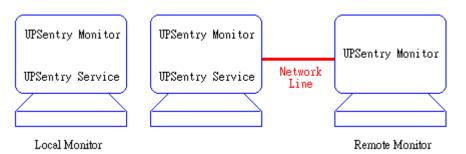
When a power event occurs, the Master gets the information then transmits it to Salve(s). Each UPSentry Service executes different "Actions"(FlexEvent) so that the system manager can configure different strategies into each different computer. For example: When a power failure occurs, the file server and mail server won't shutdown until the UPS battery is low, but other less important workstations execute
