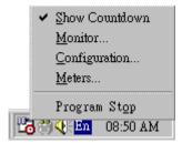
Show Countdown: UPSentry Smart 2000 displays the countdown time (time to shutdown/suspend the operating system) window to remind the user that the operating system will be shutdown or suspend in the displayed time. This function lets user know clearly how much time is left to shutdown/suspend the computer when power fails. The operating system shutdown time can be adjusted from the Action menu.
