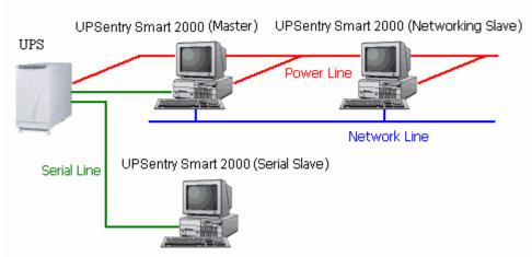
UPSentry Service can operate in "Master" Mode (which allows UPSentry Smart 2000 to send commands to its connected UPS) in "Serial Slave" mode (which listens to its connected UPS) or in "Networking Slave" mode (which obtains the UPS information from Master via the network). If two or more computers are communicating with a single UPS, only one of these computers should be in Master mode; the others should be in Slave mode to prevent them from sending contradictory commands.
